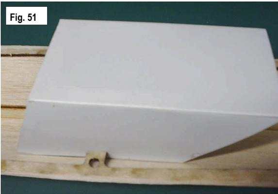
❑ **51.** The tub assembly sides should fit flush with the inside of the cockpit hatch sheeting as shown in Fig. 51.
