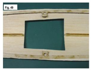
**49.** Cut the plywood frame work 1/4" back from the edge of the hatch opening as shown in Fig. 49.
