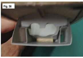
**□ 56.** The height of the seat front will be determined by the angle that the seat is raked backwards. It is only necessary to have the rear block as shown in Fig. 56.
