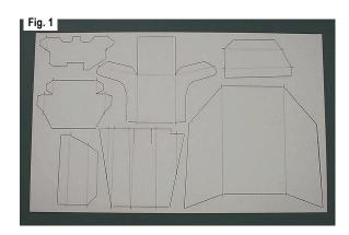
☐ 1. Use a sharp pencil or fine point marker to mark the fold lines on the laser cut styrene plastic sheet as shown in Fig. 1.
