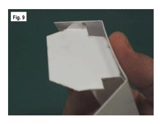
**9.** Align the bulkhead upper right tab with the rear of the tub and tack glue as shown in Fig. 9.
