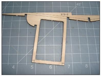
☐ 2. Use a pencil and ruler to draw a line that is 1/64" outside the inlet duct opening in B7B-2. Repeat for the other side (Photo 2)
