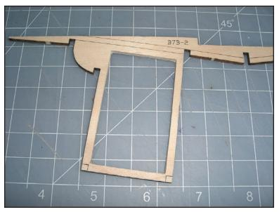
□ □ 3. Use a coping saw or a scroll saw to cut along the lines you drew earlier. Check the fit by inserting the inlet ducts into the opening.. Repeat for the other side. (Photo 3)
