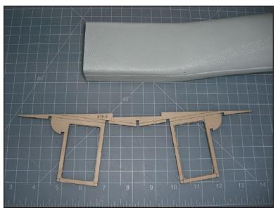
□ 1. Cut from the sheet one bulkhead B7B-2. (1/8" lite ply) Pull the inlet ducts from the poly shipping bag. Using sandpaper, gently sand the forward opening of the inlet duct to remove any excess fiberglass. Repeat for the other side. (Photo 1)
